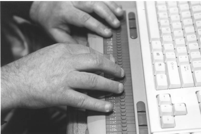
Access technology workstation: The white spots are actually tiny pegs in variable Braille keys, which individually rise and fall to form different Braille letters so the user's fingers can read what's on the screen.
